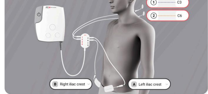
Figure 18: Example of Splitter Box and Electrode Setup
