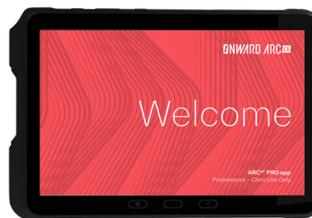
The Programmer is an off-the-shelf tablet that is pre-installed with the ARC<sup>EX</sup> PRO app and is protected by a case.
