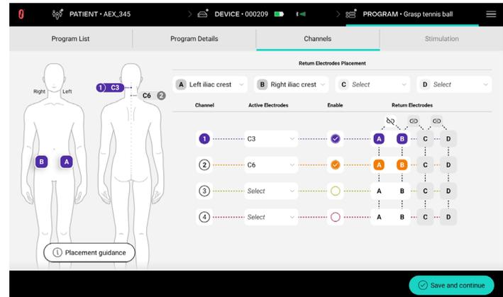
**Figure 14. Example of “Channels” Screen with recommended initial Configuration.**
