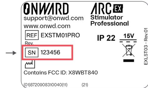
Figure 10. Example of Label on the Back of the ARC<sup>EX</sup> Stimulator.
