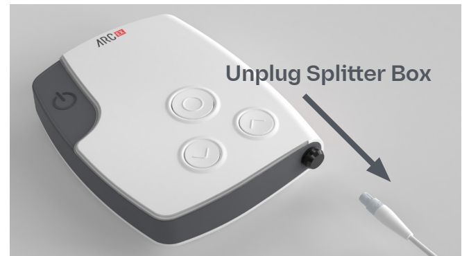
Figure 24. Prompt Interruption by Unplugging Splitter Box.
