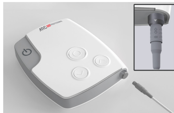
Figure 19. Connecting the Splitter Box to the Stimulator
