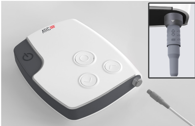
Figure 19. Connecting the Splitter Box to the Stimulator
