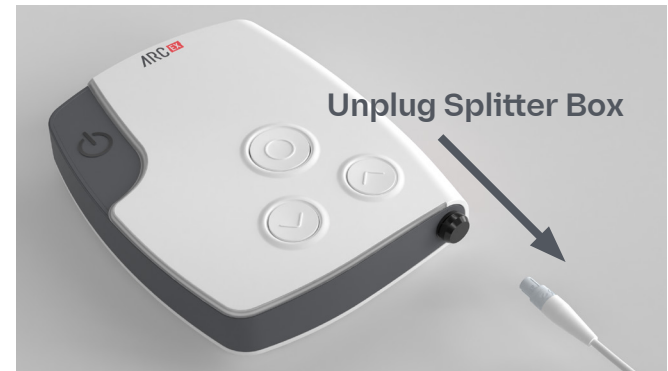
Figure 24. Prompt Interruption by Unplugging Splitter Box.
