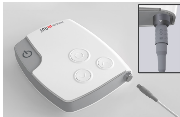
Figure 19: Connecting the Splitter Box to the Stimulator
