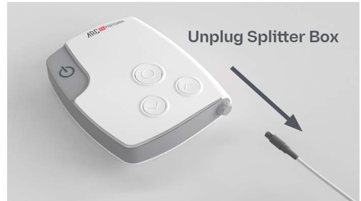
Figure 25. Prompt interruption of Stimulation by Unplugging Splitter Box,
