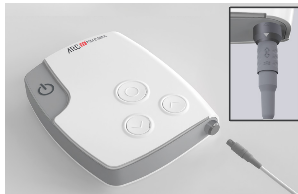
Figure 19: Connecting the Splitter Box to the Stimulator
