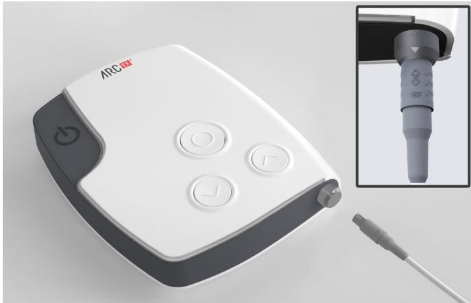
Figure 19. Connecting the Splitter Box to the Stimulator
