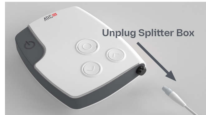
Figure 24. Prompt Interruption by Unplugging Splitter Box.
