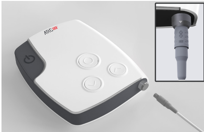
Figure 19. Connecting the Splitter Box to the Stimulator
