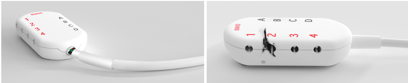
Figure 1. Examples of a damaged Splitter Box. These examples are not exhaustive.
